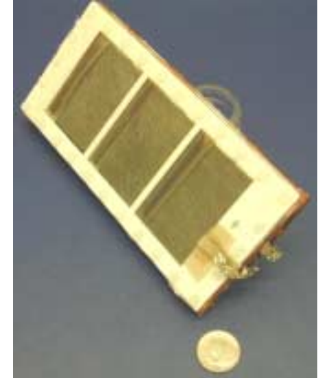
Air-Breathing "Back-to-Back" Strip Cell ('00)
