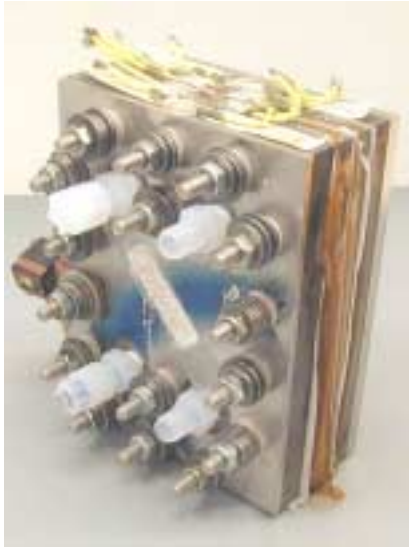
Low Pressure 25 watt Stack ('95)
